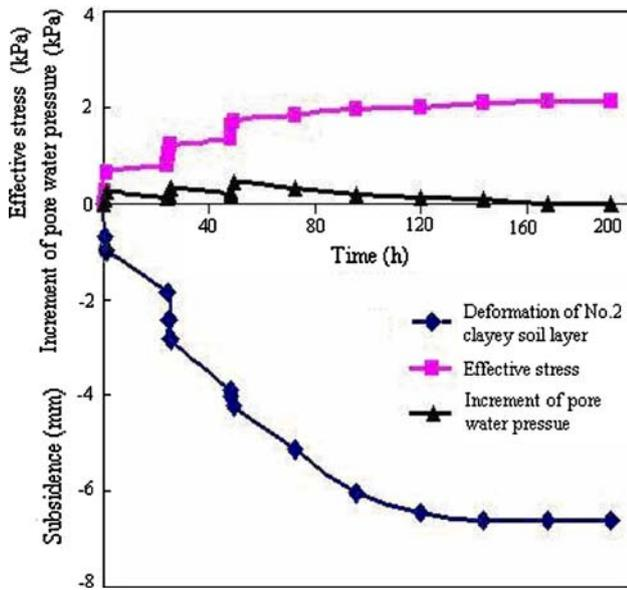
Fig. 10 Effective stress and deformation of No. 2 clayey soil layer
