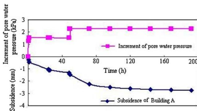
Fig. 12 Change of earth pressure and subsidence of Building A
