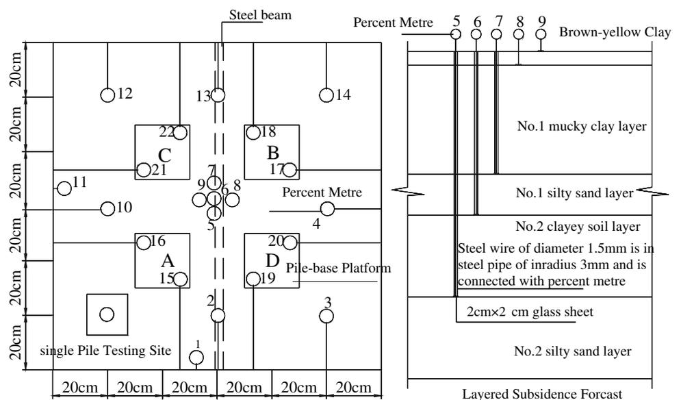
sequence for the buildings was A→B→C, D (C and D were loaded at the same time); the 3 kg counter weights being loaded for every level to simulate the construction sequence. After each loading, data from the monitoring cells were recorded. When each building had been completed, measurements were taken at intervals of 0.5, 1, 2 and 24 h and after all four buildings had been loaded, the measurements were taken every 24 h for 200 h.
