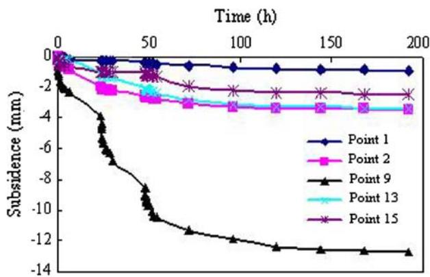
Fig. 7 Subsidence of points on the same axis
