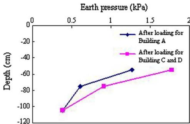
Fig. 11 Distribution of earth pressure at different depths
