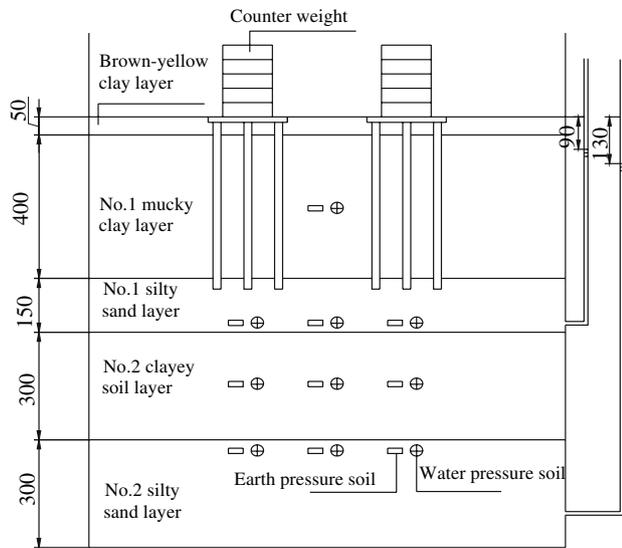
**Fig. 2** Section of model and distribution of pressure gauges (length in mm)
