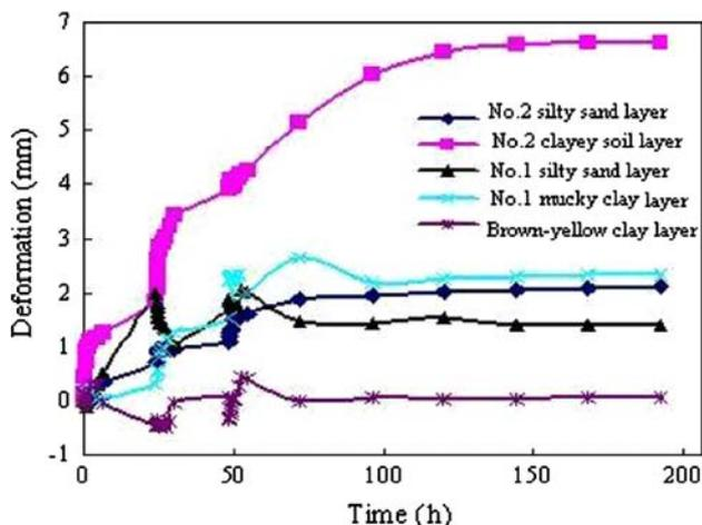
**Fig. 5** Relationship of deformation and time
