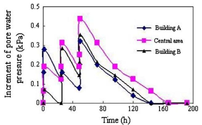
Fig. 9 Change in excess pore water pressure
